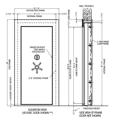
The following equipment and materials are required to install the vault door in the recommended 82" x 40" pre-formed door opening in a masonry wall of 7" thick and above.
